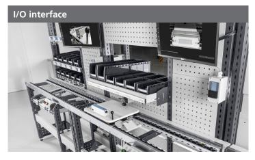
The I/O interface makes it possible to independently integrate digital inputs and outputs into the process. These can be sensors and actuators that monitor and control your process or supply it with additional information. For example, environmental conditions such as temperature or humidity could be recorded.
