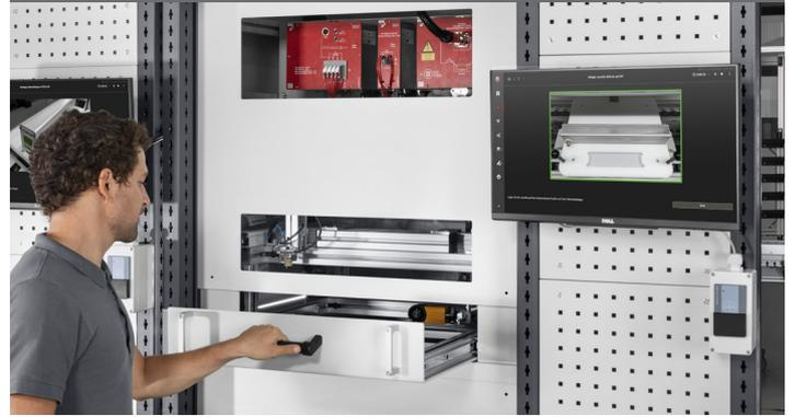
The Vision Interface enables you to automatically inspect components. In this way, faulty wiring or assembly of components can be detected using camera technology and the passing on of an incorrectly assembled product can be avoided.
